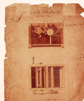
Eli Whitney's original cotton gin patent drawing
